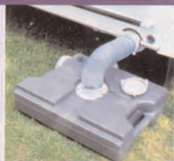
ABOVE: Large lock-on flexible pipes complete the sealed waste system LEFT: An enclosable shower area and a stainless steel basin feature in the washroom
