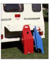
Our unique water management system provides probably the neatest and yet simplest solution to fresh and waste water management available enabling the caravan to be operated from either mains fresh and waste water supplies or alternatively from wheeled fresh and waste water containers which store conveniently in the rear boot.
